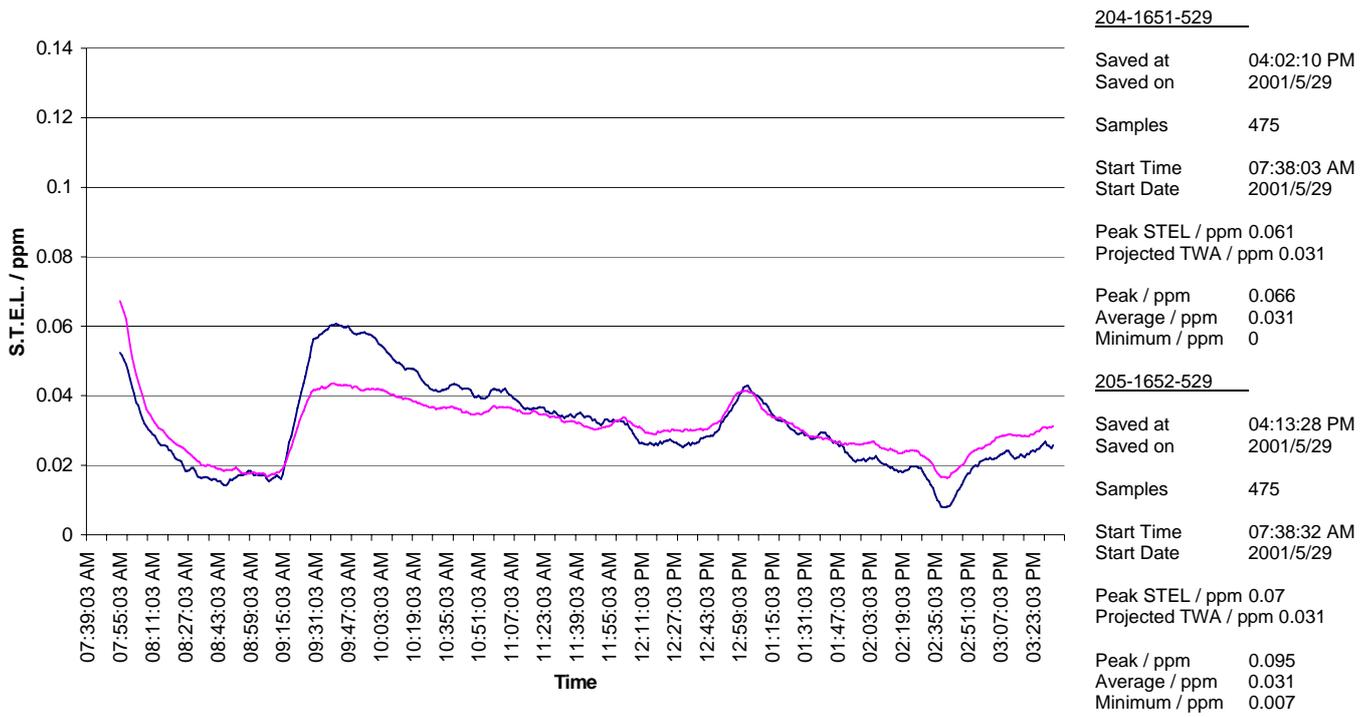
**Figure 1 - IAQ(1P, 8H) Profiles on Formaldehyde and Profile Statistics of An Office by Two Units of PPM Formaldemeter**
